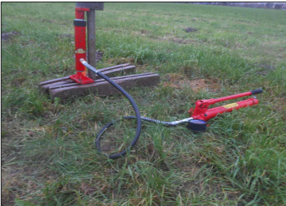
Image 2: vertical pull-out test
