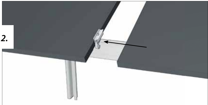
Fig. 6.1.-2. (pushing/sliding the module to the clamp)
